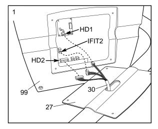
2. Attach the Console (99) to the Handrail (27) with the four Small Screws (6). Make sure that the Handrail Wire Harness (not shown) is not pinched between the Console and the Handrail.
